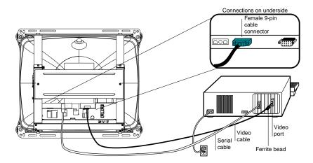
• Connect the touchscreen cable. Connect one end to the appropriate port on the back of your computer. Connect the other end of the cable to the touchscreen connector on your touchmonitor. The touchscreen cable connectors should fit snugly into the connectors on your touchmonitor and computer. Secure the cable by turning the thumbscrews on each connector.
